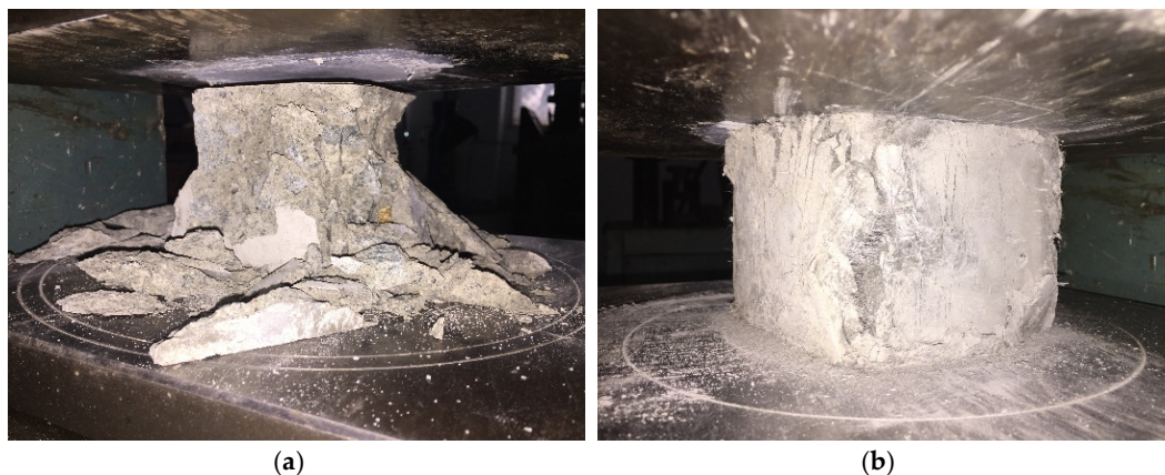
Figure 4. Compressive failure modes of cubic specimen. (a) Reinforced concrete (RC) cubic specimen. (b) PP-ECC cubic specimen.
