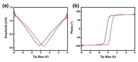
Fig. 3 (a) The standard ferroelectric amplitude curves. (b) The phase curves obtained by applying a ramp voltage from -6 to +6 V.
