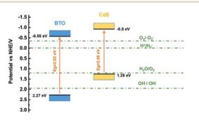
Fig. 9 Schematic band structure of the CdS/BTO NWs samples.
