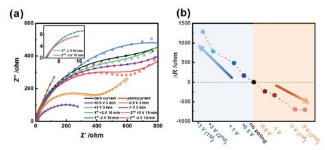
Fig. 5 (a) EIS Nyquist plots of the CdS/BTO NWs samples after different polarizations and the inset shows the results for  $-3 V (1^{st})$  and  $-3 V (2^{nd})$ . Open circles were test data points and solid lines were corresponding fitting. (b) Impedance change value compared to unpolarized sample of the CdS/BTO NWs samples.
