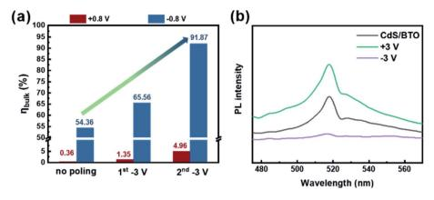
Fig. 6 (a)  $\eta_{\text{bulk}}$  of the CdS/BTO NWs samples after different polarizations, (b) PL spectra of CdS/BTO NWs after different polarizations.
