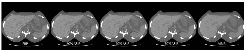
FIG. 2. For illustration purpose, images of the Kyoto Kagaku phantom acquired at 3 mGy CTDI_{vol} and reconstructed with the three different algorithms: FBP, ASiR, and MBIR.
