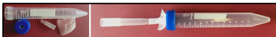
Figure 4. Homemade tube for removing liquid from larval or floating tissues. Some larval and adult tissues float in solution during fixation. This simple tool consists of a nylon mesh held by a 200 \mu L cut tip, followed by a 1 mL tip as an adaptor to connect to an aspirator. Liquid can be safely removed without losing any tissue. Please click here to view a larger version of this figure.
