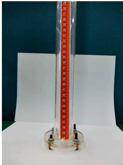
Figure 5. FBG pressure sensor unit installed at the bottom of a liquid container.
