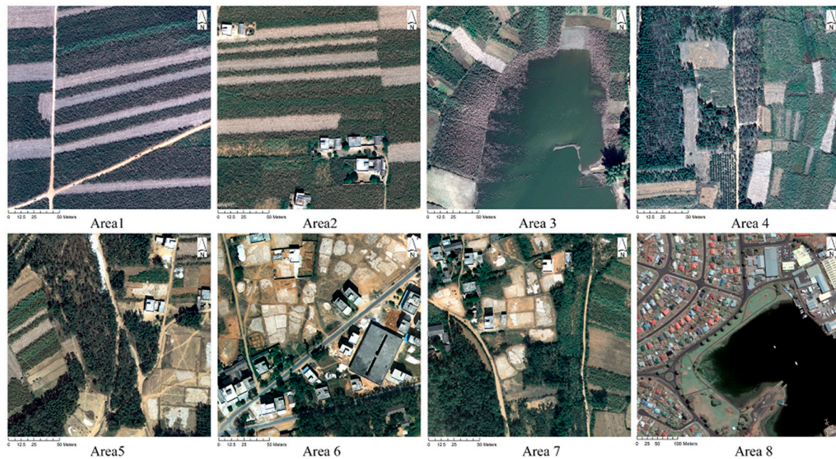
Figure 2. Study areas. Areas 1 to 7 are aerial images with 3 bands (R: 610–660 nm; G: 535–585 nm; and B: 430–490 nm), Area 8 comprises GeoEye-1 images with 4 bands (R: 675 nm; G: 545 nm; B: 480 nm and NIR: 850 nm). Each area is limited to 1000 \times 1000 pixels. Therefore, the numbers of positive samples are limited to within 1.1% of the whole population (0.3%, 0.5%, 0.6%, 0.5%, 0.6%, 0.6%, 0.7%, and 1.1%, respectively).
