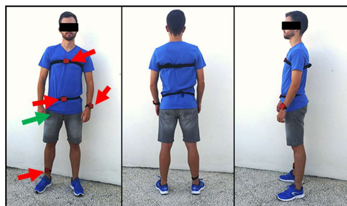
Figure 2. Example of the distribution of the sensors worn by an experimental subject. The green arrow indicates the position of the smartphone. Red arrows correspond to the SensorTag modules, which are attached to the user's body by means of elastic bands.
