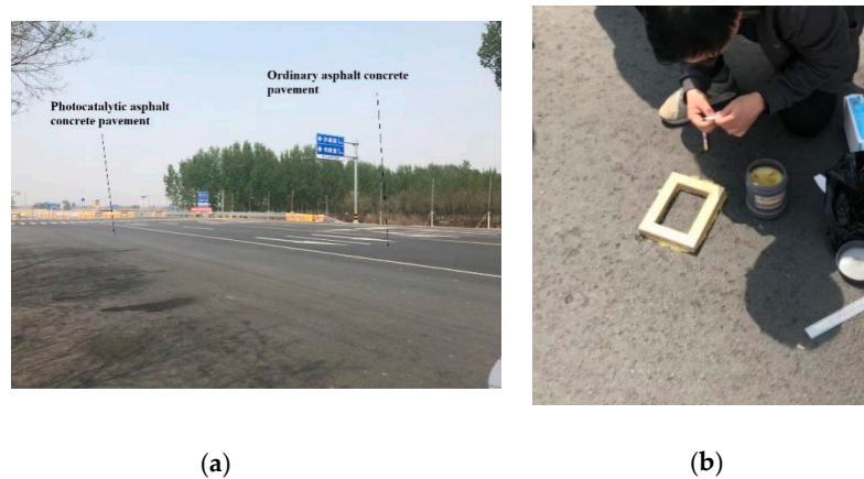
Figure 10. Outdoor nitrogen oxide collection experiment: (a) photocatalytic pavement and original pavement; (b) collecting water samples.
