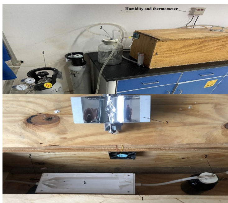
Figure 2. Test system; external (above), internal (below). (1) Reaction mold; (2) Running-in interface; (3) Probe; (4) Nitrogen dioxide bottle; (5) Cover plate; (6) Flow rate control; (7) Xenon lamp.
