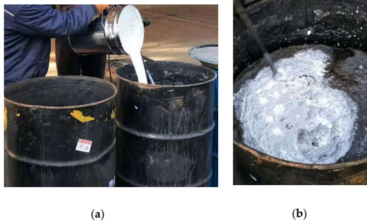
Figure 8. Preparation of functional Sand-fog seal: (a) adding; (b) mixing.
