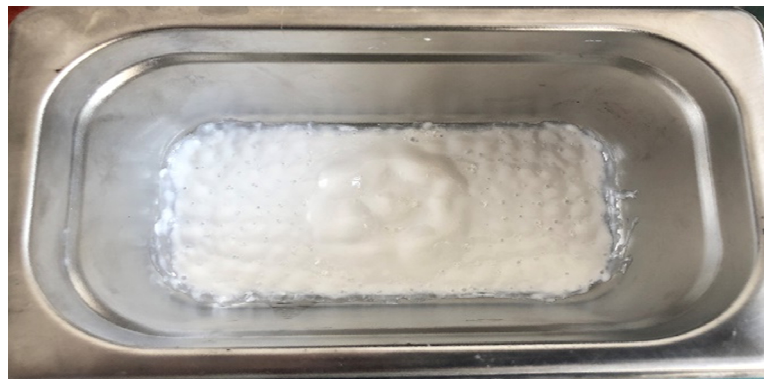
Figure 4. Ultrasonic vibration of titanium dioxide.
