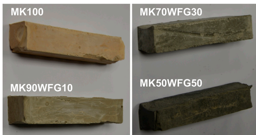
Figure 4. Appearance of the 28-day cured specimens.
