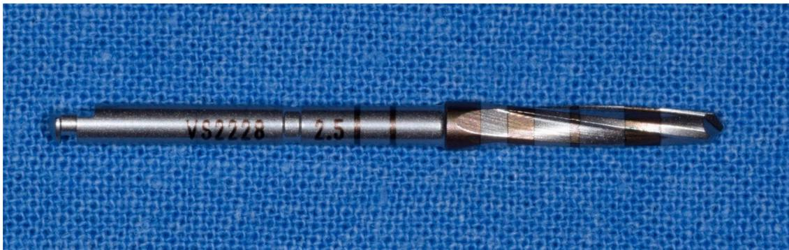
**Figure 8.** Fourth cutter with a diameter of 2.5 mm in the method “implant drilling with bone compaction instrumentation technique.”
