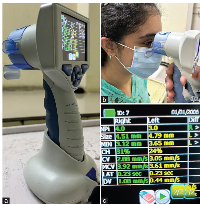
Figure 2: An image of neurological pupil index-200 (NeuroOptics Inc., Irvine CA, USA) pupillometer device along with smart guard and charging station (a); an image of measurement being carried out (b); output of various pupillary parameters measured on the result screen by the device (c)
