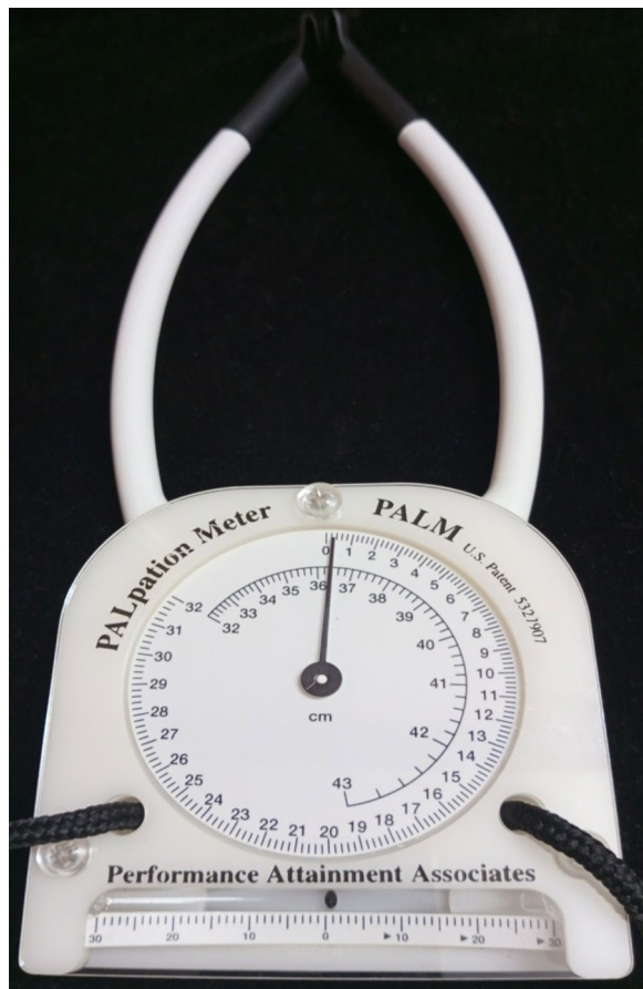
Fig. 2. The pelvic inclinometer (PALM) with an inclinometer and two caliper arms.
