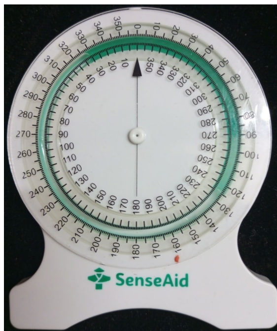
Fig. 3. The bubble inclinometer, a rounded plastic inclinometer with a 360 rotating dial and fluid indicator.
