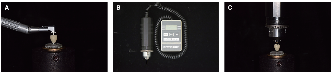
Fig. 3. (A) Tightening the abutment screw with an insertion torque of 20 Ncm using a hand torque wrench. (B) Digital torque gauge used in this study. (C) Removal torque value measurement using the digital torque gauge.
