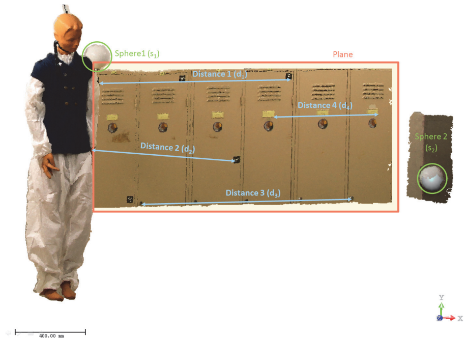
Fig 6. Dimensional analysis based on distances measured between ground control points (artificial targets) and basic primitives (spheres and planes) fitted in the first crime scene.
