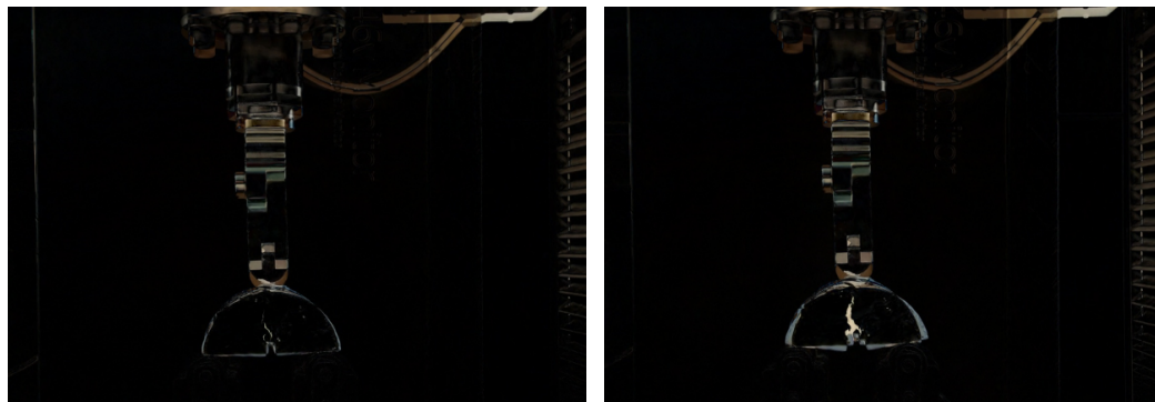
(a) S1 specimen crack initiation stage
