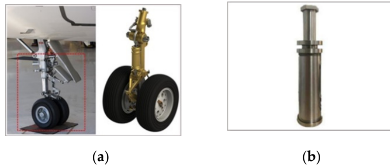
Figure 21. Hydraulic parts. (a) Application of hydraulic parts in aircraft landing gear. (b) The tested hydraulic part.
