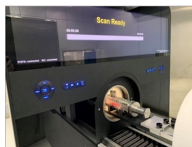
Figure 23. Scanning the hydraulic part.
