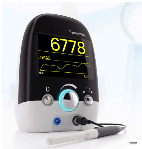
Figure 4 Sentimag® Localization Platform showing the handheld magnetic probe connected to the console which displays the relative intensity of the signal (Endomagnetics Ltd., Cambridge, UK) (67).
