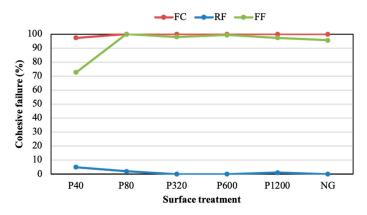
**Figure 11.** Cohesive failure percentage of the adhesive joints under different surface treatments with the adhesion promoter.
