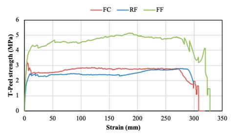
Figure 14. Characteristic T-peel stress-elongation curves of the 3 PSAs.
