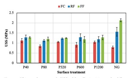
**Figure 5.** Ultimate shear strength (USS) of the adhesive joints under different surface treatments without adhesion promoter.
