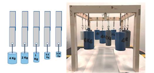
Figure 3. Creep tests illustration and setup.
