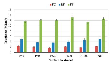
Figure 13. Toughness of the adhesive joints under different surface with the adhesion promoter.
