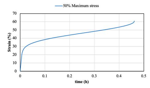
Figure 16. Characteristic creep curve of the FF under the 50% of the maximum shear tensile value.
