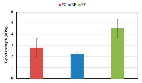
Figure 15. T-peel strength of the PSAs (NG condition with the adhesion promoter).
