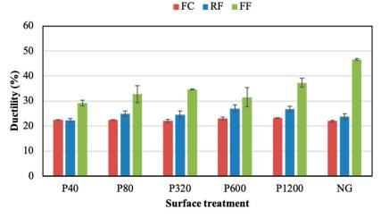
Figure 7. Ductility of adhesive joints under different surface treatments without adhesion promoter.
