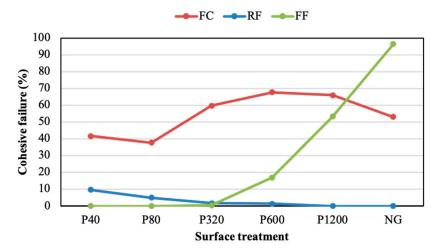
**Figure 6.** Cohesive failure percentage of adhesive joints under different surface treatments without adhesion promoter.
