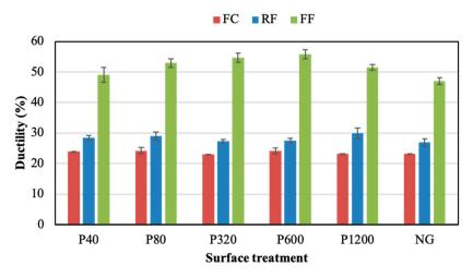
Figure 12. Ductility of the adhesive joints under different surface treatments with the adhesion promoter.
