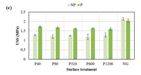
**Figure 10.** USS values of joints with (P) and without (NP) adhesion promoter for aluminium joints assembled with (**a**) FC, (**b**) RF, and (**c**) FF.
