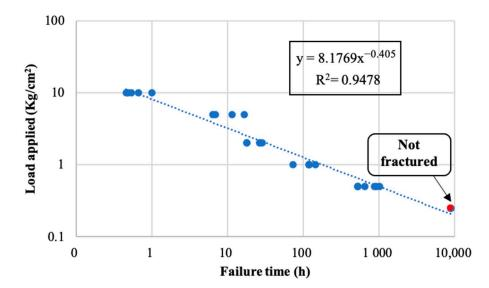
Figure 17. FF adhesive fracture time for the different loads applied.
