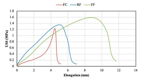
Figure 4. Characteristic shear stress-elongation curves of the 3 PSAs.
