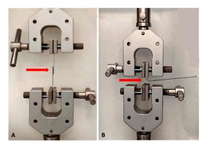
Figure 2. Example of adhesive shear (A) and T-peel (B) tests.
