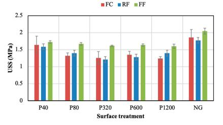
Figure 9. Ultimate shear strength (USS) of adhesive joints under different surface with adhesion promoter.
