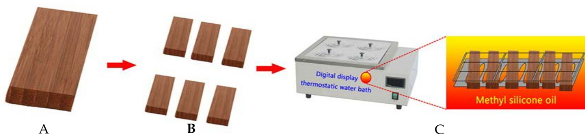
Figure 7. Schematic diagram of hot oil treatment. (A) Bamboo scrimber. (B) Saw cutting. (C) Hot oil treatment.
