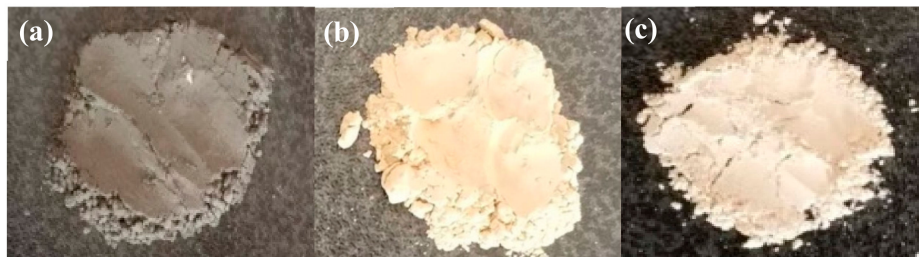
Figure 11. Whiteness pictures of (a) fly ash (FA), (b) CFA, and (c) ZCFA powders.
