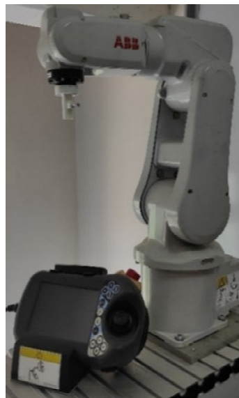
Figure 6. 6-degree of freedom industrial robot arm.
