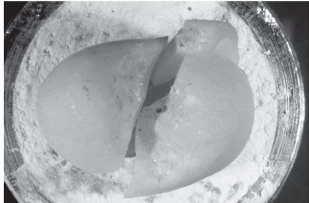
**Figure 3-** Fractured specimen after application of compressive load
