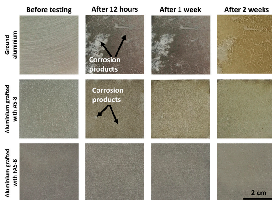
Figure 9. The surface appearance of ground aluminium and treated aluminium surface with AS-8 and FAS-8 after selected exposure times in the salt spray chamber, test performed according to standard ASTM B117-19, i.e., 5 % NaCl, 35 °C.
