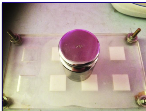
Figure 2: Pouring the room-temperature-vulcanized silicone elastomer material into the mold with a constant load (1 kg) placed over the acrylic mold.
