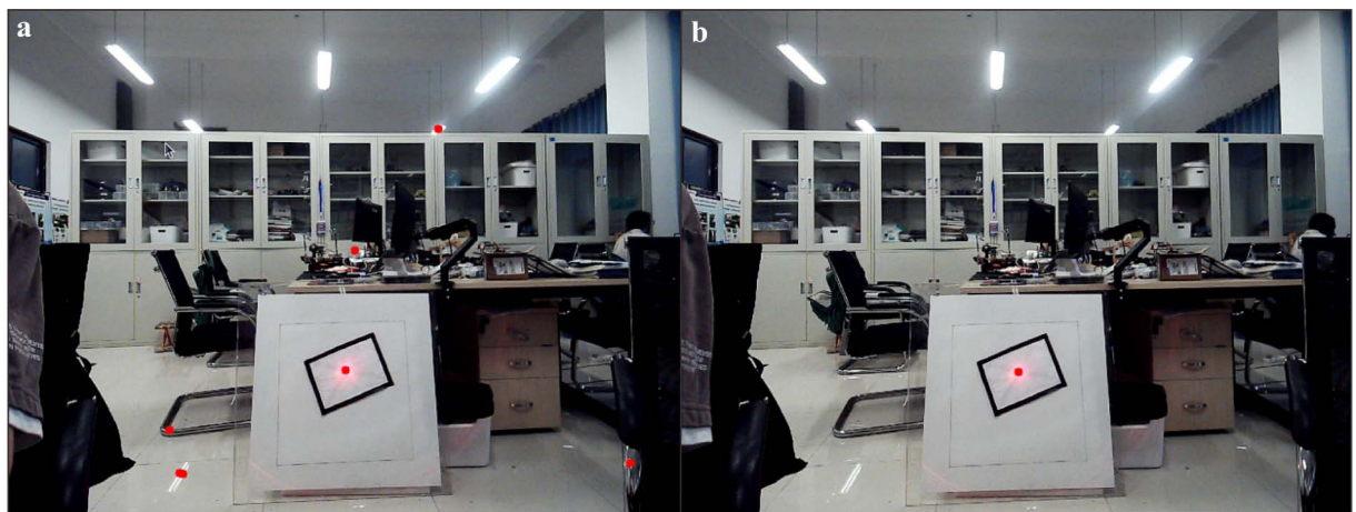
Fig 8. Interference in the laboratory environment. (a) Any area of high brightness identified as a potential laser spot. (b) The effective laser points identified after mitigating interference through the application of constraint conditions.
