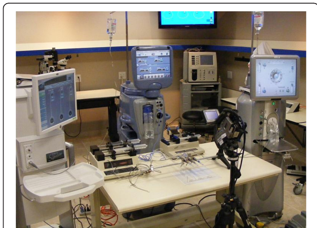
Figure 1 The basic experiment setup. The thermal imaging camera, surrounded by 3 phacoemulsification units.
