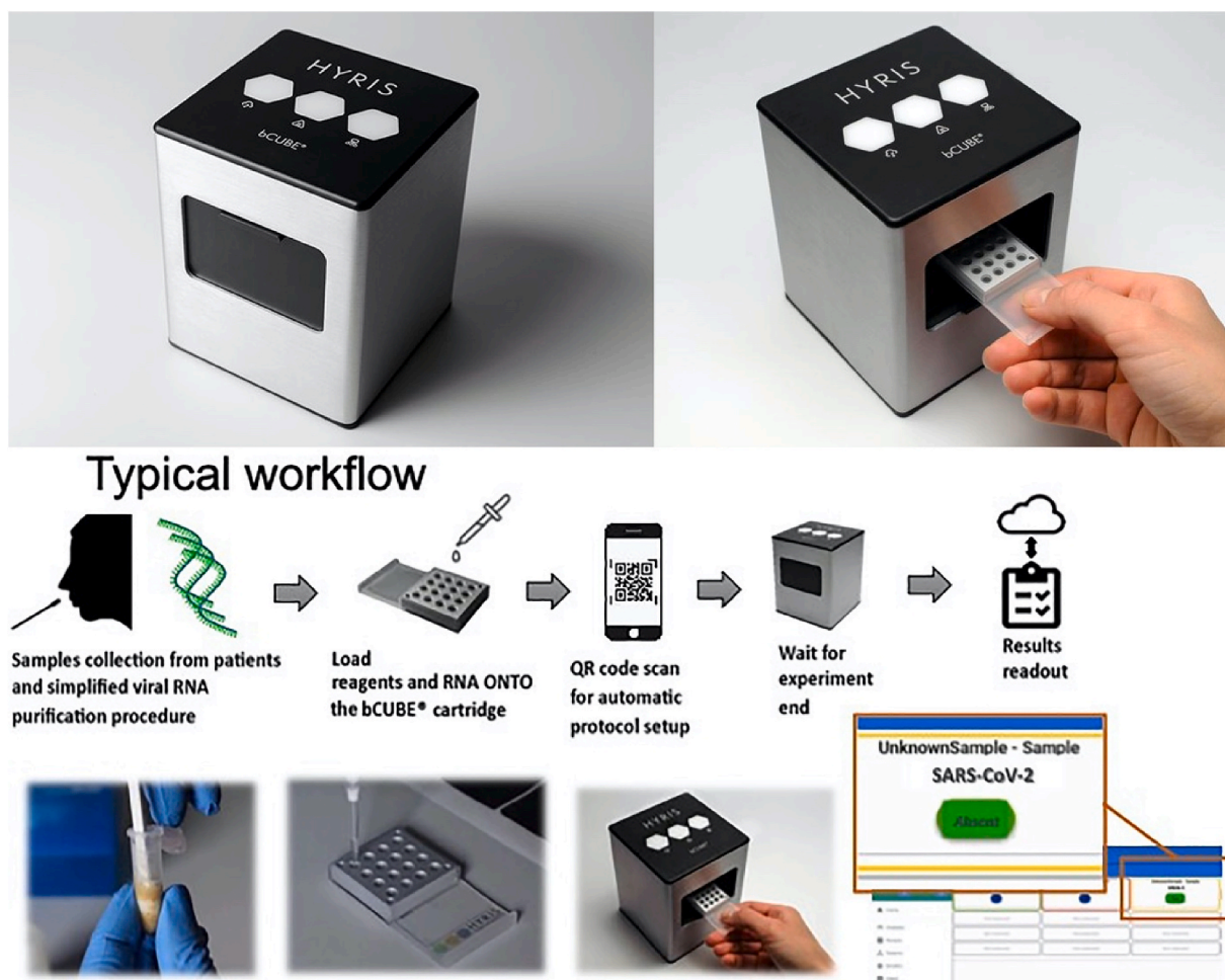
Fig. 2. Portable PCR device bCUBE® and how it is used. Reproduced with permission from Ref. [65]. Copyright 2020 John Wiley and Sons.
