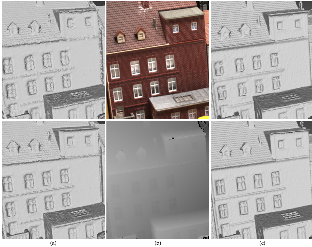
Figure 8. Object edges in the reconstructed meshes, the original image and the depth map. From left to right: (a) the object edges in surface meshes reconstructed by the method in [5] (top) and our method (bottom) without the dense visibility technique; (b) the original image and the corresponding depth map with a similar view point; and (c) the object edges in surface meshes reconstructed by the method in [5] (top) and our method (bottom) with the dense visibility technique.
