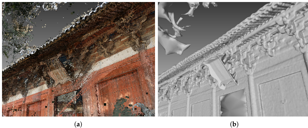
Figure 1. An example of the application of the proposed method in the field of cultural heritage digitalization, (a) point cloud; (b) mesh.
