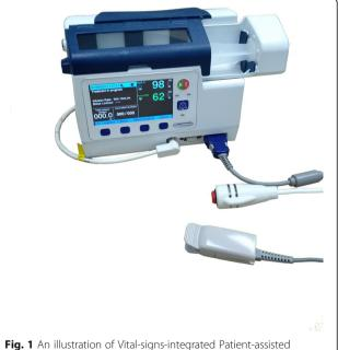
**Fig. 1** An illustration of Vital-signs-integrated Patient-assisted Intravenous opioid Analgesia (VPIA) analgesic infusion pump. The algorithm and the VPIA analgesic infusion pump ("Intellifuse pump"; Model: Opiva) was designed by Innovfusion Pte Ltd., Singapore. The written permission has been given for publication by Innovfusion Pte Ltd., Singapore
