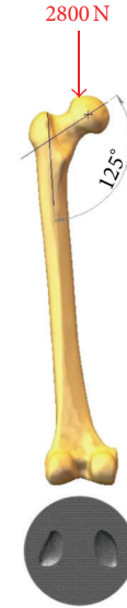
FIGURE 1: The femoral models were aligned in neutral upright configuration and were loaded with a simplified vertical force of 2800 N. All models were distally supported on the same fixed tibial component model.
