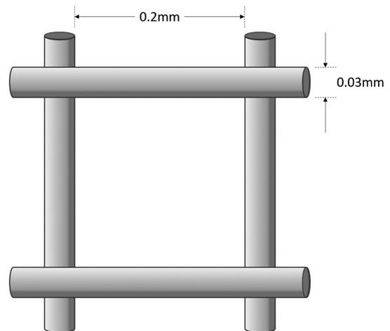
$$\text{Metal coverage ratio (\%)} = \{ 1 - ( 0.2 \times 0.2 ) / ( 0.23 \times 0.23 ) \} \times 100 \approx 24.4$$
