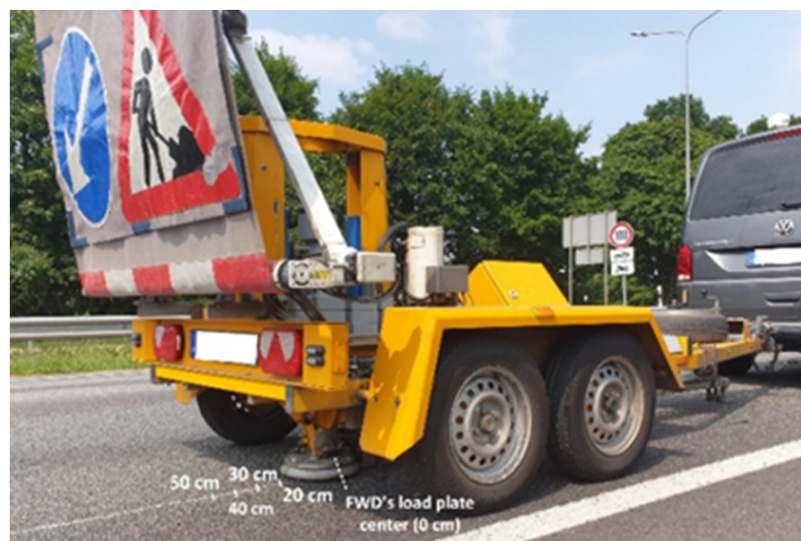
Figure 4. Realization of FWD experiments for calibration purposes of the embedded optical sensors.
