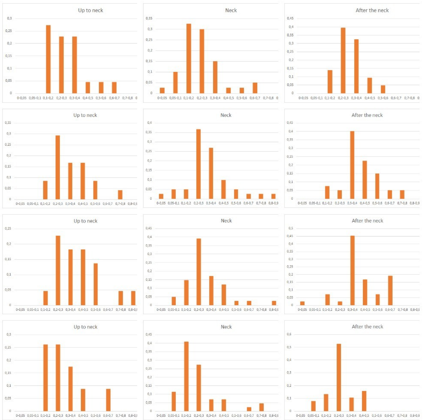
Figure A2. Histograms of \Delta WSS distribution over the stent surface of Patient 2.
