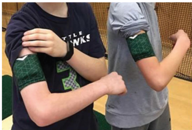
Figure 1. Inertial sensor and depiction of placement during game-day collections. The sensor was secured using a modified protective wrist/forearm guard placed 3 to 5 cm above the lateral epicondyle of the throwing arm. The sensor weighs about 16 g and is approximately 3.5 × 3.5 × 1 cm in size.
