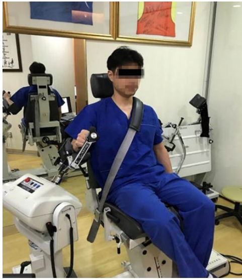
Figure 2. External rotation exercises were carried out with the shoulder at 20° of abduction and forward flexion. The participant sat on the dynamometer with the trunk fixed by a cross seat belt.
