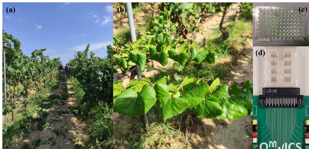
Figure 1. Grapevine leafroll disease and grapevine fanleaf disease diagnosis by ELISA and lab-on-a-chip (LOC) assays to detect Grapevine leafroll-associated virus 3 (GLRaV-3) and Grapevine fanleaf virus (GFLV). (a,b) Grapevines affected by GLRaV-3; (c) ELISA assay with diluted virus sources (1:3, 1:5, 1:10, 1:20, 1:50 and 1:100); (d) developed platform for portable, on-field LOC assays, with the sensor inserted in the PCB platform, ready to be connected to the potentiostat. Tests were carried on different dilutions (1:10, 1:20, 1:50, 1:100 for GLRaV-3 or 1:5, 1:10, 1:20, 1:50, 1:100 for GFLV).
