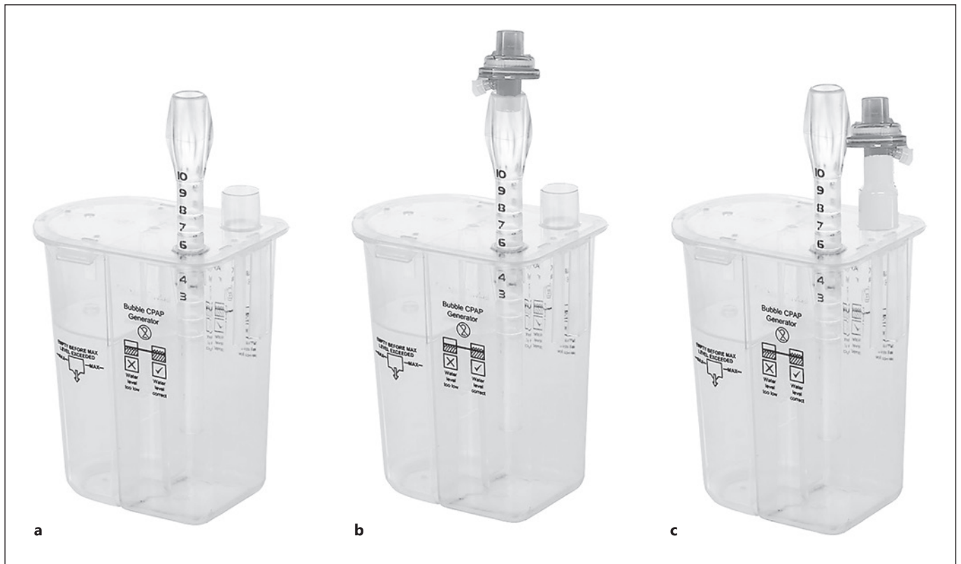
Fig. 1. Filter placement. Control, standard setup (a); pre-generator expiratory limb (b); and post-generator at point of flow exit into environment (c).
