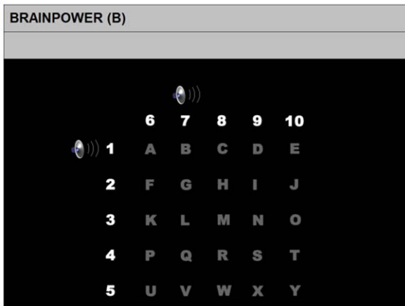
Figure 1. Visual support matrix displayed on a computer screen to the participant during the auditory P300-BCI experiment [22]. The matrix was identical to the visual P300 BCI matrix. The speakers displayed at the top left corner of the matrix indicate the auditory presentation of numbers and were not displayed during the actual experiment. doi:10.1371/journal.pone.0053513.g001
