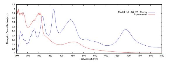
**Figure 9.** Comparison between the calculated spectra for the Model 1-d structure (blue line) and the experimental absorption of a 0.25mg/mL solution of DHI in EtOH (red line, curve corresponding to the absorbance after 600 min).
