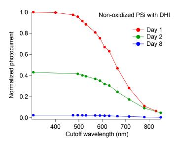
**Figure 1.** Normalized photocurrent measurements obtained in three different days on the same PSi/eumelanin sample.
