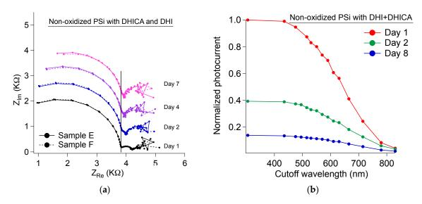
**Figure 5.** Behavior of PSi/eumelanin samples prepared using a 50/50 DHI/DHICA mixture. (a) GEIS measurements; (b) normalized photocurrent measurements.
