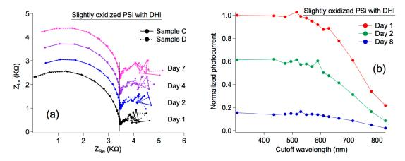
**Figure 3.** Behavior of PSi/eumelanin samples with a slight surface oxidation (3%, as defined in the text) of PSi before impregnation. (a) GEIS measurements; (b) normalized photocurrent measurements.
