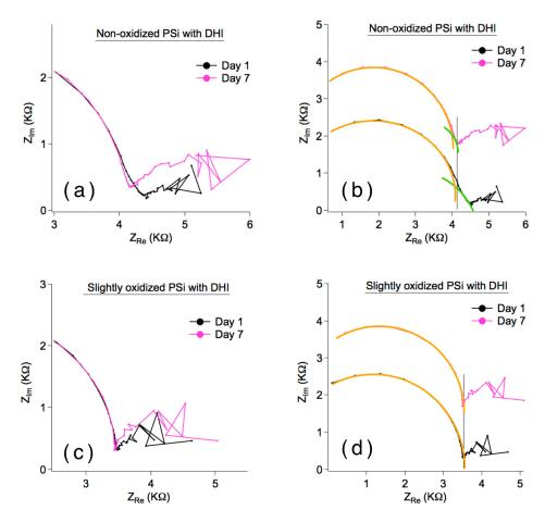
**Figure 4.** Graphical analysis of the GEIS results of Figure 2 (panels (**a**,**b**) and of those of Figure 3a (panels (**c**,**d**)). The results of the first and seventh days are shown. In panels (**a**,**c**) are reported the enlarged views of the data of Figures 2 and 3a, respectively. In panels (**b**,**d**) partial ellipses are used as a visual guide to show the presence of an additional resonance in the non-oxidized samples (**b**) with respect to the slightly oxidized samples (**d**).
