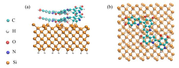
**Figure 10.** Adsorption of two stacked tetrameric models 1-d by Panzella [48] on a Si surface. The full system with the slab of the surface supercell used in the calculations is displayed: (a) side view; (b) top view. The bottom atoms are hydrogen-passivated.
