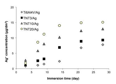
Figure 9. The cumulative silver release profile obtained on the basis of ICPMS data.
