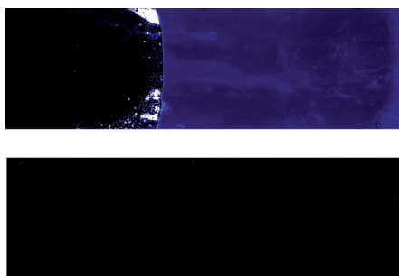
Figure 7. Scan images of amino-functionalized slide prior to (bottom) and after reaction with 5 (top; the part of the slide shown on the left was not functionalized to facilitate handling) as described in the text; \lambda_{\text{exc}} = 488 nm, \lambda_{\text{em}} = 550\text{--}600 nm (standard green filter in emission), photomultiplier tube (PMT) voltage = 500 V.
