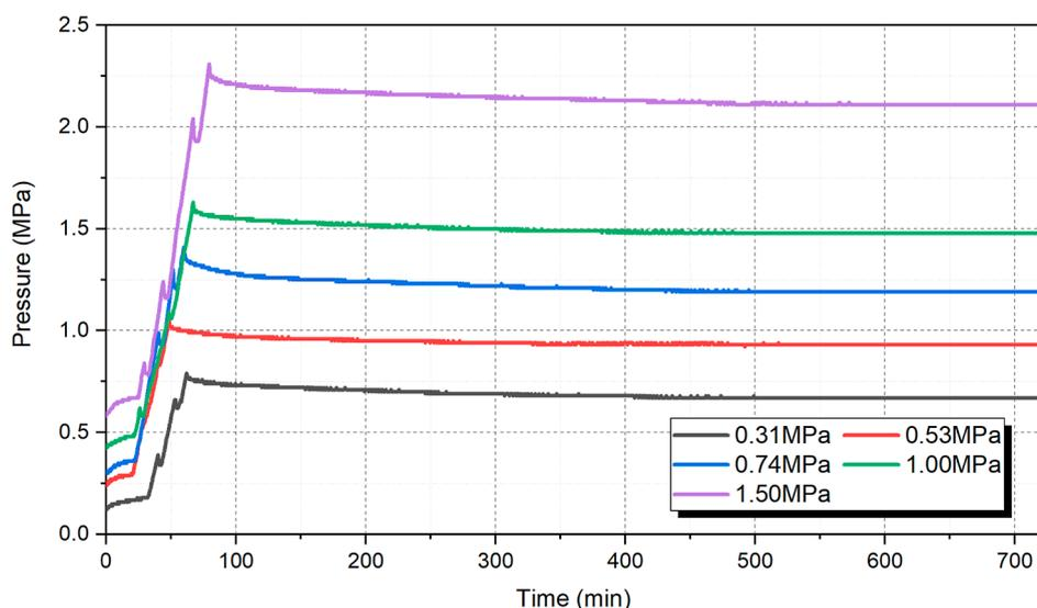
Figure 10. Comparison of pressure recovery curves under the contact water injection mode.
