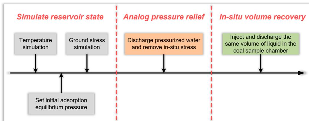
**Figure 8.** Experimental procedure of *in situ* volume recovery by contact injection.
