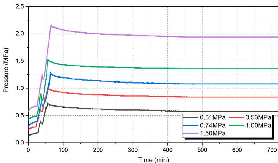
**Figure 14.** Comparison of pressure recovery curves under the contact oil injection mode.
