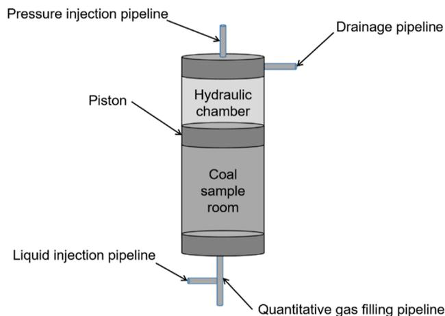
**Figure 7.** Schematic diagram of the coal sample tank.
