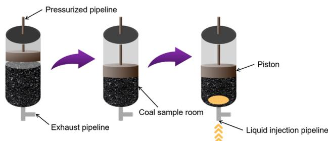
**Figure 5.** Legend of stress loading and contact liquid injection combination experiment.
