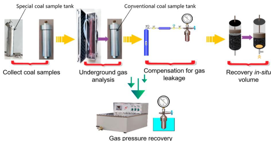
Figure 2. Technical route of the non-seal gas pressure measurement technology.
