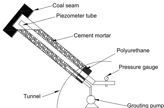
Figure 1. Direct measurement of coal seam gas pressure.
