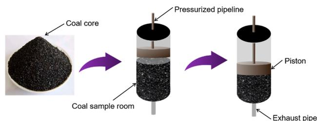
Figure 4. Schematic diagram of compressed free space.
