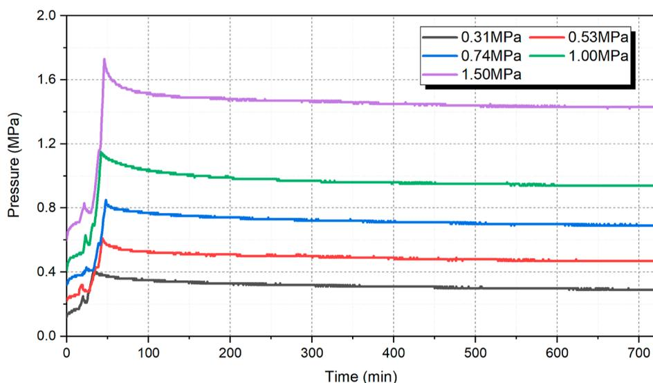
Figure 17. Comparison of pressure recovery curves under contact oil injection/stress loading.
