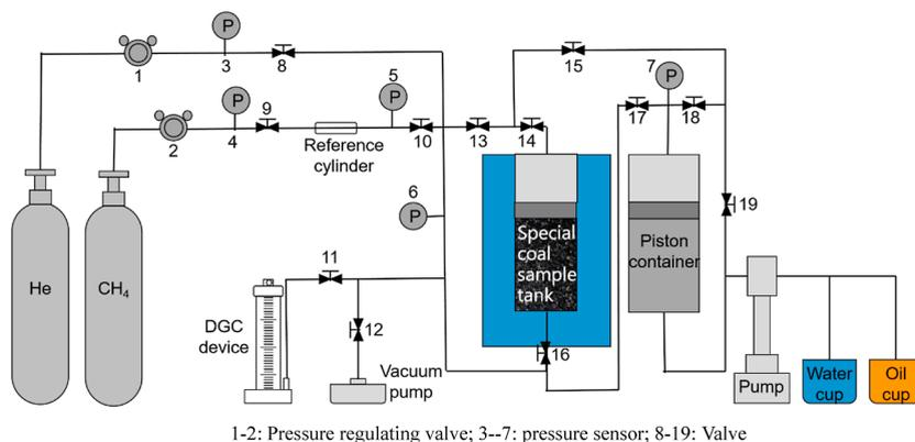
1-2: Pressure regulating valve; 3--7: pressure sensor; 8-19: Valve
