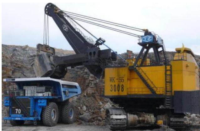
(a) The way of unloading material of electric shovels.
