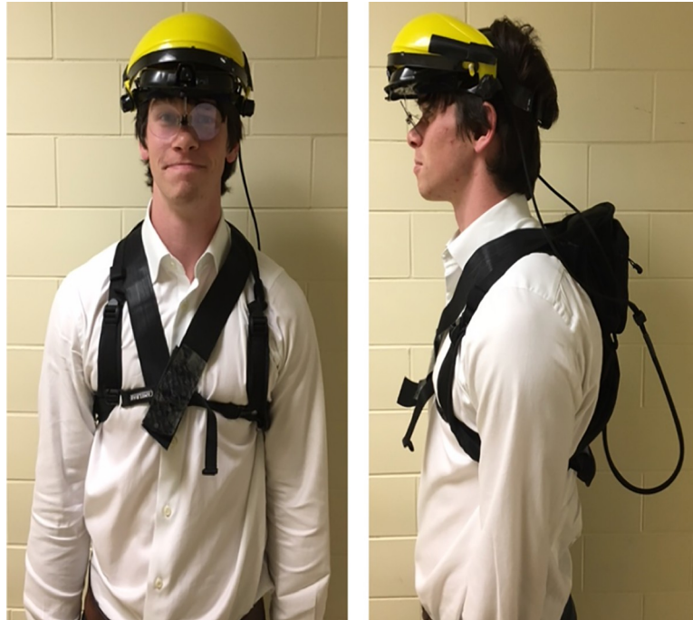
Fig 2. ISCAN Omniview-TX Head-Mounted Eye tracking device worn by one of our authors (MC). This has been modified by combining it with a face shield (portion in yellow), allowing the glasses to be held tightly against the face even while moving. In addition, the transmitter was placed into a backpack, which allowed for a natural place for the transmitter to be housed while an individual was running.
