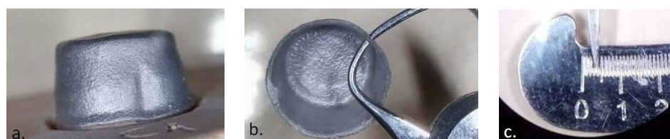
Figure 5. (a) CAD Software screen view of the 3D copy framework design; (b) external surface of Co–Cr copy framework; (c) the thickness of the copy wall measured with a mechanical micrometer; (d) the scale of the instrument indicated a thickness of 35 \mu\text{m} .
