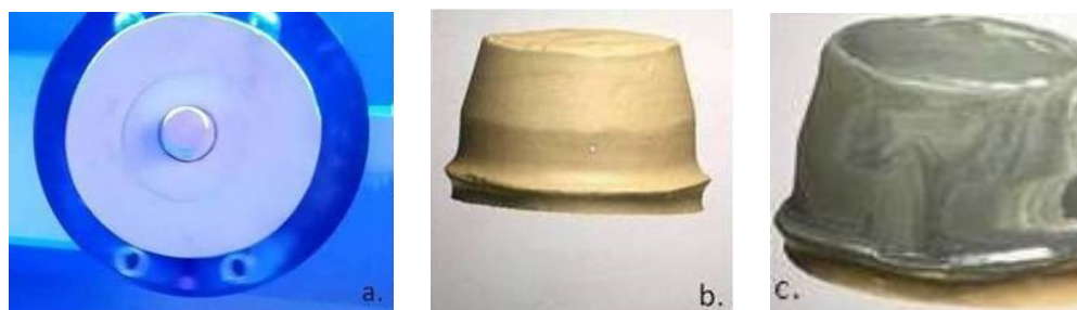
Figure 4. (a) Scanning of the dental laboratory stone cast using structural blue light; (b) computer-aided design (CAD) software screen view of a digitalized dental cast (abutment); (c) CAD software screen view of the 3D coping framework design.
