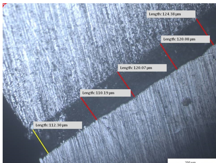
Figure 16. Micrographic segment (200×) after measuring the length of the gap between removable partial denture framework and mucosal area at the V1 area (V1—area, segment d6).
