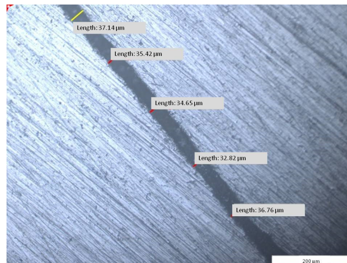
Figure 14. Micrographic segments ( 1000\times ) after measuring the length of the gap between the joined frameworks of the dental prosthetic frameworks assembles (I1—area 1, segment g2).
