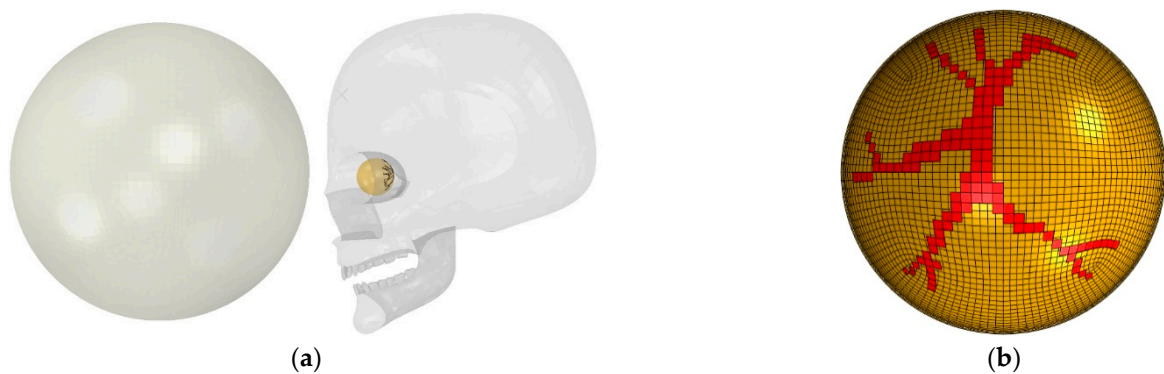
Figure 2. Finite element model of soccer ocular injuries. (a) Initial setup of a flying soccer ball hitting the face, including the eyeball; (b) retinal vessels in the posterior retina (frontal view).
