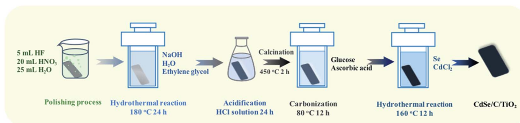
Scheme 1 Preparation processes of the CdSe/C/TiO 2 nanofiber film.
