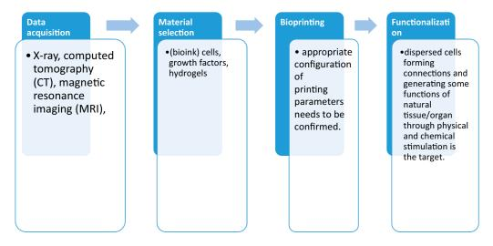
Figure 1. Illustrating the stages involved in the process of tendon bioprinting.
