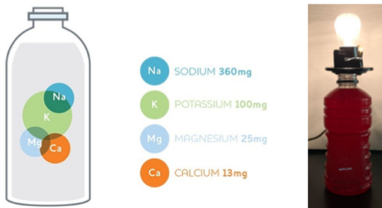
Figure 1. Electrolytes in sports drinks cause light bulb illumination
