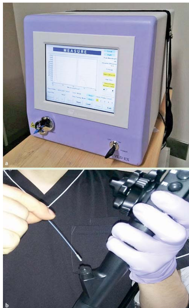
Fig. 1 a VLD-EX exposes the colorectal tumors to light using a special probe-type fiber. b Special probe-type fiber was inserted from the channel of the endoscope.
